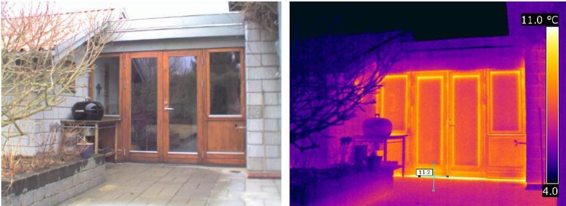
**Figur 4.** Gable (west) with window to the bedroom. This room's outer wall was previously insulated from inside. However, a thermal bridge interruption was omitted along the floor concrete slab and therefore the socket shows orange on the thermography to the right. The U-value was measured to 1.03 (Id 19) compared with the insulated outerwall U-value=0.32 (Id 22), see Table 1.
