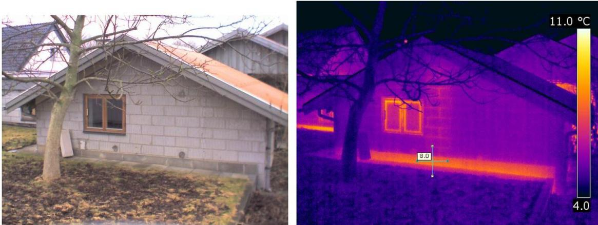
At the thermography on figure 5, the dark shaded areas also represents cold surfaces, but with *low* heat insulation. The low insulation gives rise to low surface temperatures inside. The yellow and orange areas represent better insulated areas and therefore capable to keep the heat inside the room which in turn results in higher surface temperatures.
