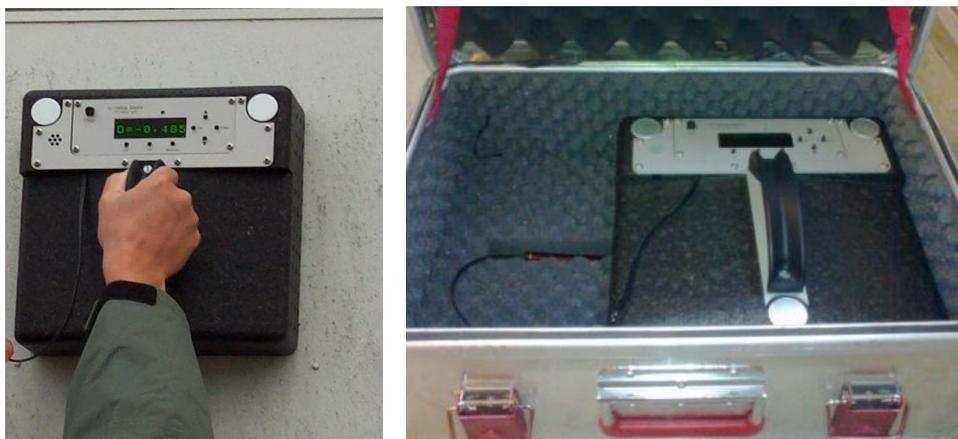
This apparatus is based on a principle where the heat is 'trapped' by a heat absorption sensor (copper plate) when it leaves the outdoor surface of the test piece. A copper plate is used, as the absorption sensor due to its high thermal diffusivity and high conductivity [2,3].
