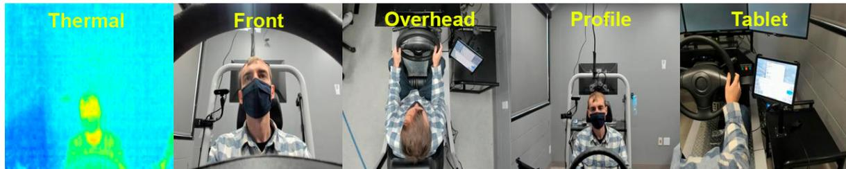
**Figure 2.7.** The five views of the driver: overhead view, face view, thermal view, profile view, and tablet view. The first three views represent the driver-center views, while the last two views represent a view for entry pose analysis and tablet-related features.
