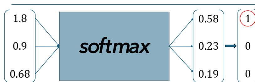
FIGURE 2.13: Softmax activation transfer process. Example values given in text section. Own illustration
