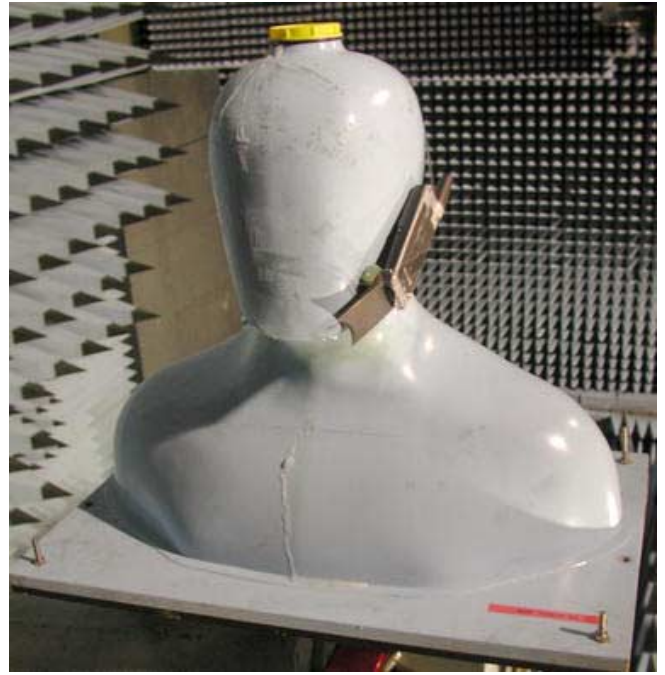
Figure 1. A handset mounted on the head/shoulder phantom.
