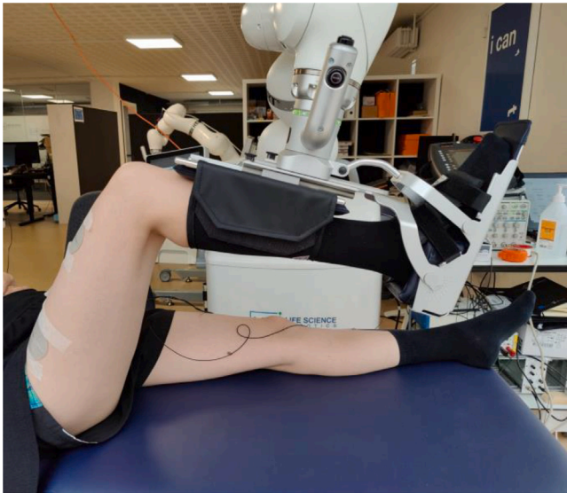
Fig. 1. ROBERT ® is a seven-degree-of-freedom robotic manipulator that can move the lower limb of a patient in a lying position. The participant's leg was attached to the end effector of ROBERT ® through a foot brace.
