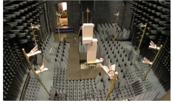
Figure 2. Setup used in the MIMO OTA testing.
