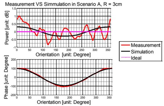
Figure 7. Simulation and measurement comparisons for single plane wave with AoA = 0 degrees in terms of power and phase variations at radius 3cm
