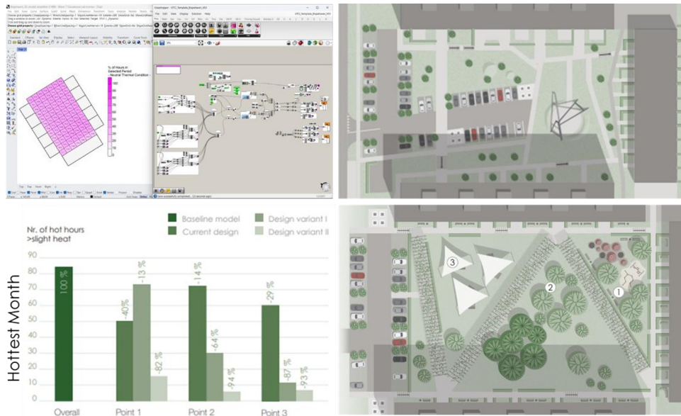
Fig. 1. Insight to case study 1 simulation-based design workflow regarding outdoor comfort. Top left: Simulation environment in VPL. Top-right: current site condition. Bottom left: heat stress performance comparison of 3 design variants. Bottom right: simulation environment in VPL.
