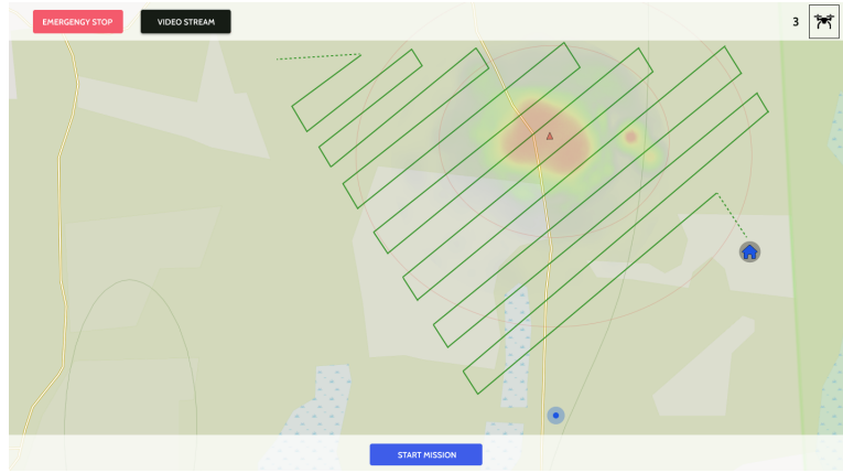
Figure 4: Map with a heatmap layer generated through the lost person model. Darker colors denote higher probability of detection of person in that area.
