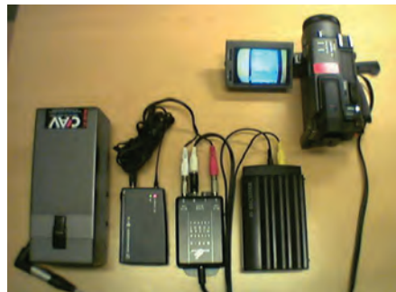
Figure 10. Observer (left) carrying and operating portable audio/video equipment (right) for capturing high-quality data in the field.
