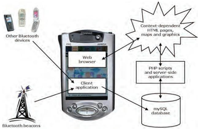
Figure 3. Just-for-Us prototype system architecture.
