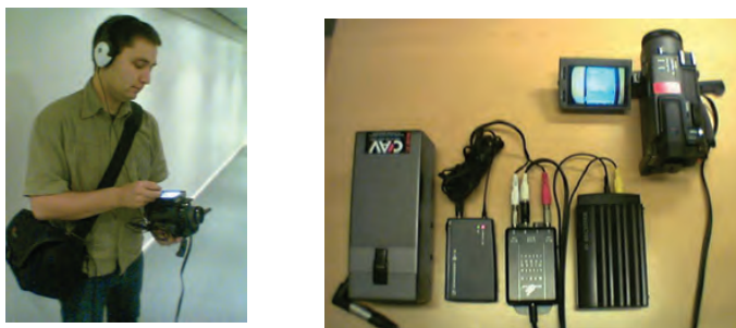
Figure 17. Observer (left) carrying and operating portable audio/video equipment (right) for capturing high-quality data in the field.
