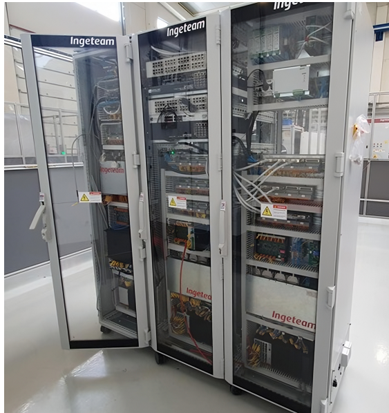
(a) Hardware-in-the-Loop (HiL) platform.
