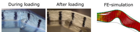
Fig. 11. Wrinkle at the top transition during loading (left), after the load is removed (centre), and in the FE-simulation (right).
