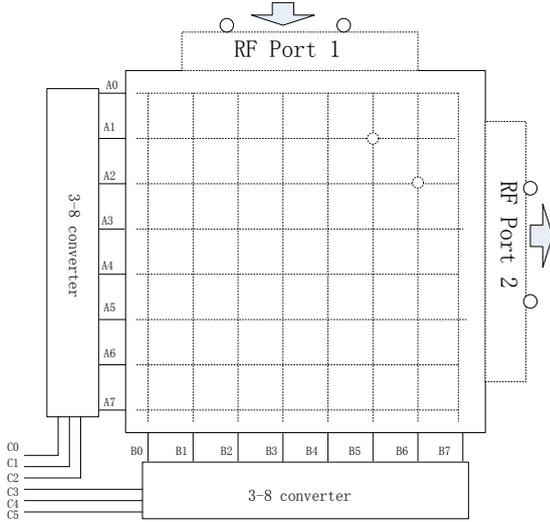
Fig. 3 Topology of address-searching network for 64 patterns switching.
