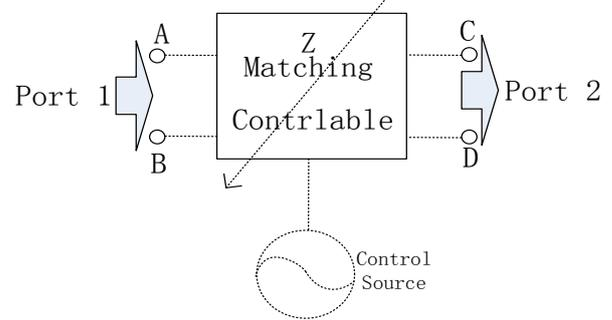
Fig. 2 Topology of a signal controlled Matching network.
