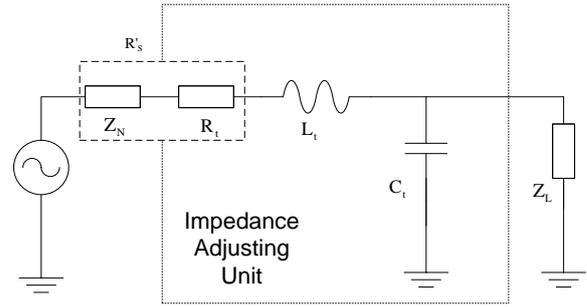
Fig. 4.A smallest matching unit inside the adjusting network.
