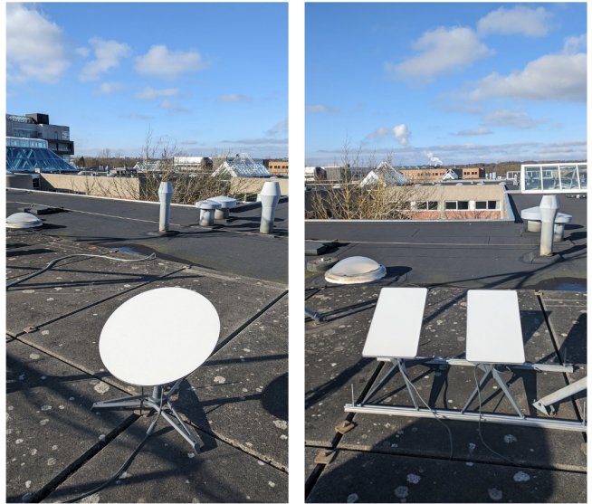
Fig. 1. Starlink antenna configuration used to obtain the experimental data: one Gen-1 (left) and two Gen-2 (right) Starlink Standard Actuated antennas.
