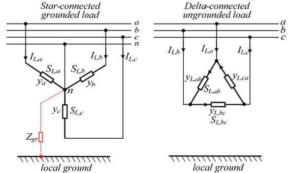
Fig. 6. Wye (left) and delta-connected (right) spot loads
