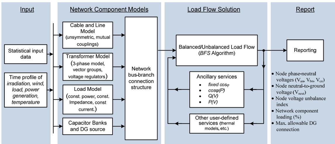
Fig. 1. Generalized functional block diagram of the load flow method developed in Matlab<sup>®</sup>
