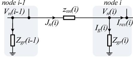
Fig. 5. Closer look on the neutral and grounding circuit. Current directions are matched with Carson's circuit
