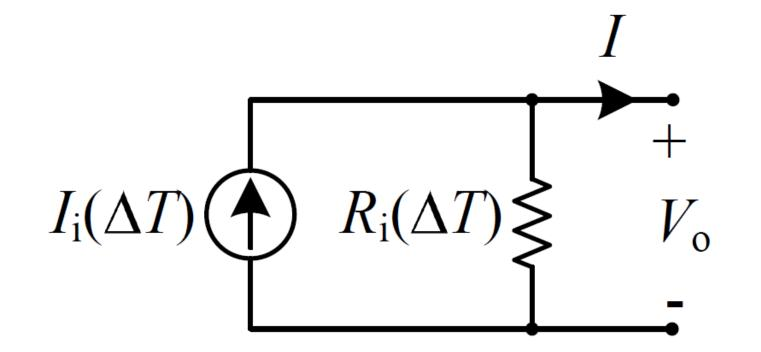
The inner voltage source, current source and resistance depends all on the temperature difference  $\Delta T$  [°C] of the module.
