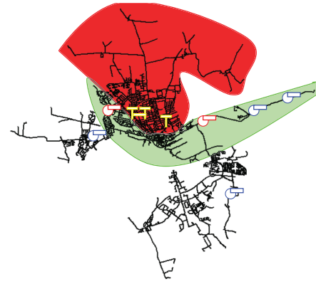
Fig. 3. WDN of Randers. The pumping stations to be controlled are shown in red and the remaining in blue. Tanks are shown with a “T” shaped symbol in yellow.
