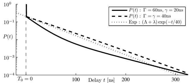
Figure 3. Delay-power intensity of the S-V model (solid line). The parameter values of  $\Lambda, \lambda, \Gamma, \gamma$  correspond to the estimates reported in [3]. The dashed curve correspond to the selection  $\Gamma = \gamma = 40\text{ns}$ . For comparison, the dotted curve provides a purely exponential decay.
