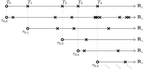
Figure 1. Realization of Poisson point processes corresponding to the S-V model. Circle points indicate fixed delay components. The top process occurs with rate  $\Lambda$  while each of the lower processes occurs with rate  $\lambda$ . A new point process is initialized whenever a new point emerges from the top process.
