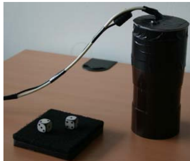
Fig. 2 The Gamble system. The preliminary version allowed for interactions by the use of handheld devices. The current version employs a camera mounted cup of dice and a speech recognition system to capture the users input.
