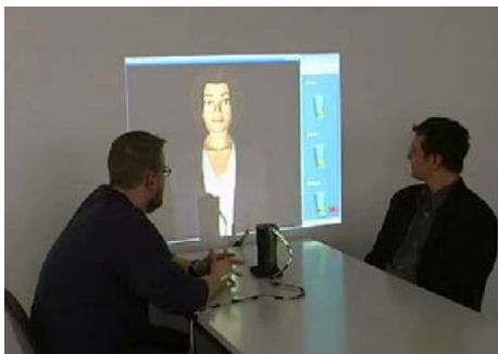
Fig. 2 The Gamble system. The preliminary version allowed for interactions by the use of handheld devices. The current version employs a camera mounted cup of dice and a speech recognition system to capture the users input.
