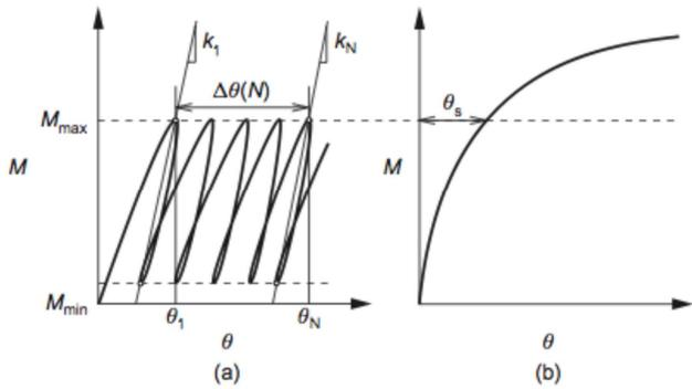
Fig. 9 The rotation as function of number of load cycles. (LeBlanc et al. 2010)
