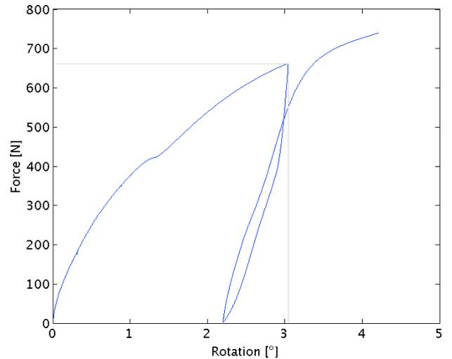
Fig. 4 The force-rotation relationship in the static test with failure determined at 3°.
