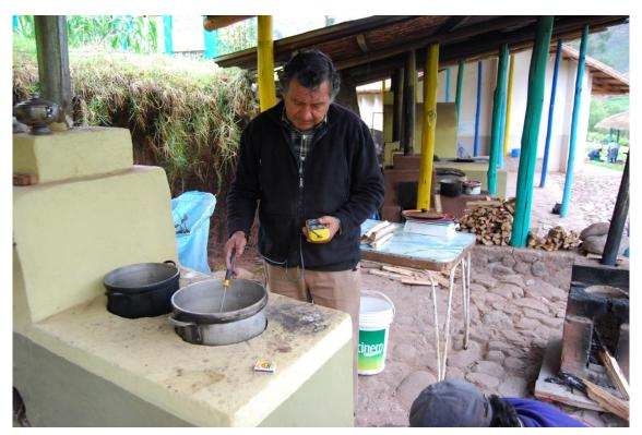
Improved cooking stove Nina (Peru) have a thermal efficiency of 30% and new efficient wood cooking stove IDER (Brazil) saves 40% of solid-fuels
