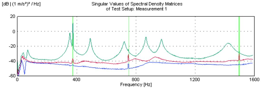
Figure 6. Indication of harmonic components at 374 Hz, 748 Hz and 1496 Hz in the SVD plot.
