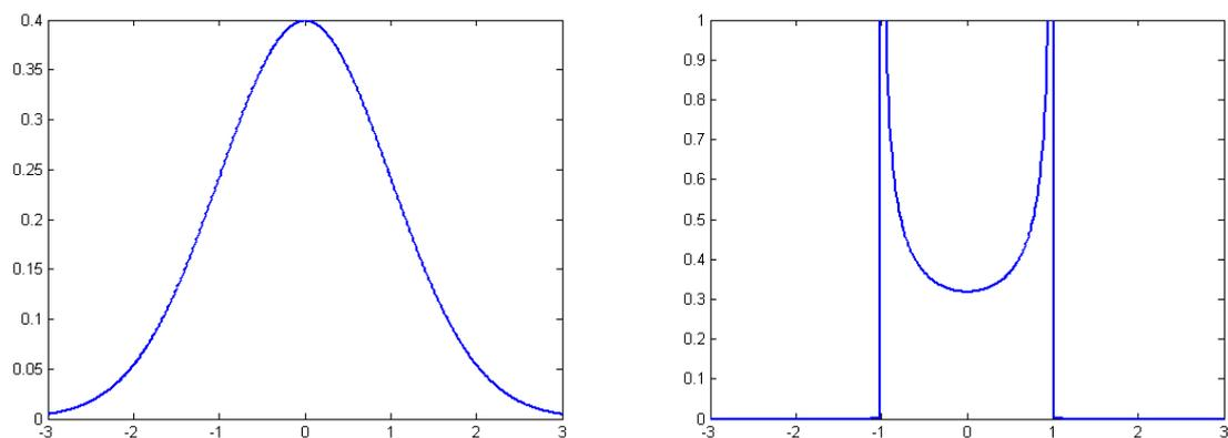
Figure 1. Normalized PDF of pure structural mode (left) and pure harmonic component (right)
