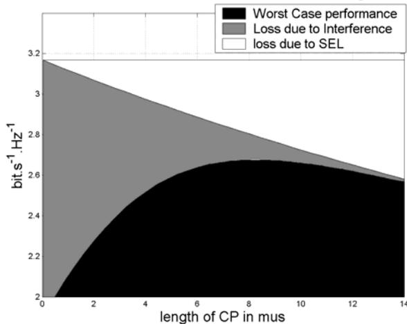
Figure 6: On the efficiency of the CP to cope with multipath, Exp3000, SNR=20dB,  $T_s = 60\mu$ s.
