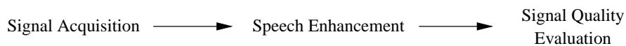
Figure 1.2: The work flow of a speech enhancement development cycle. The signal acquisition could consist of controllable, simulated signal generation. The speech enhancement method is the device under test, and evaluation is a toolbox of tools to evaluate the quality of improvement by applying the speech enhancement method.
