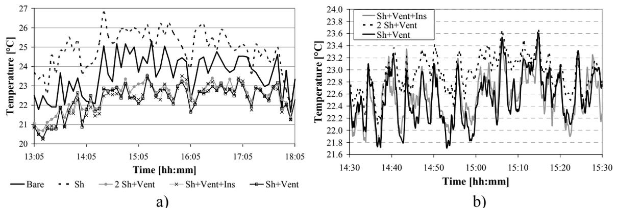
Figure 6. a) Measured air temperature for the 5 tested solutions, reported as 5 minutes average values. b) Measured air temperature for the ventilated thermocouples.
