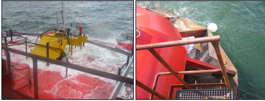
Fig. 3.2 Heel of 10° to the front. This leaves the base-plate uncovered
