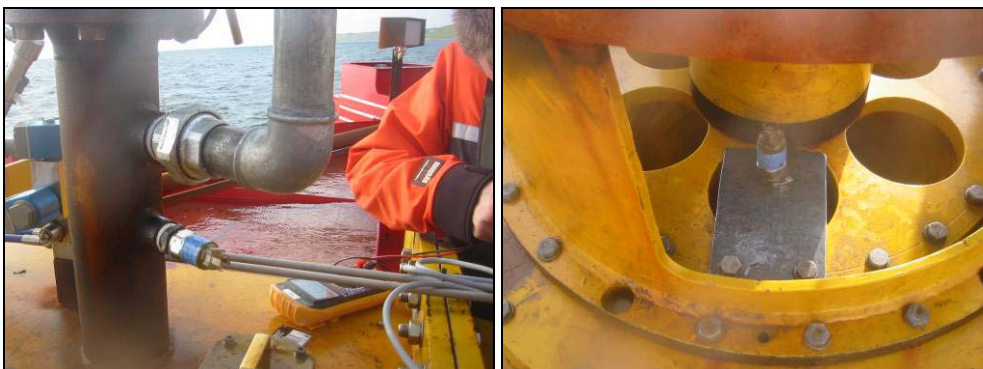
Fig. 4.1 Aeration tube water level switch installation and siphon turbine water level switch.
