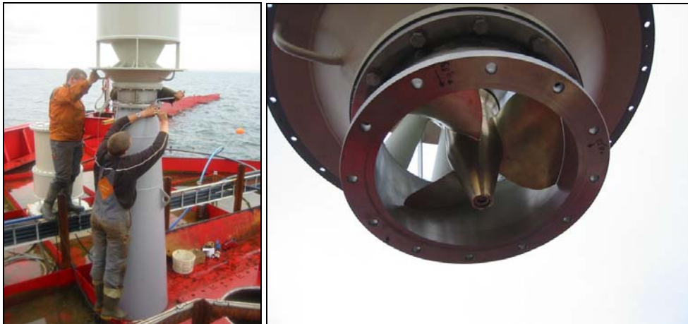
Fig. 4.12 Draft tube & centre section assembly and turbine runner
