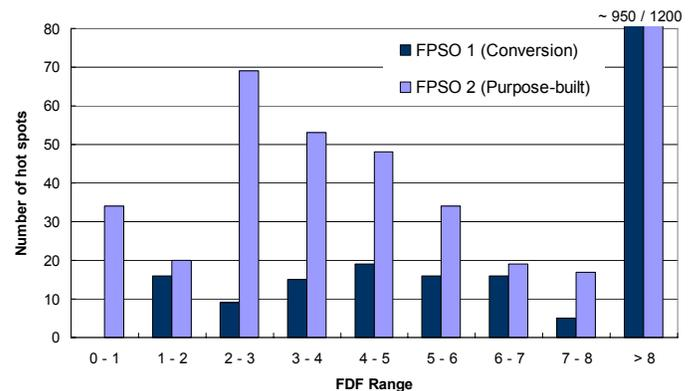
Figure 6. Distribution of *FDFs* observed in 5 different tanks on 2 FPSOs.
