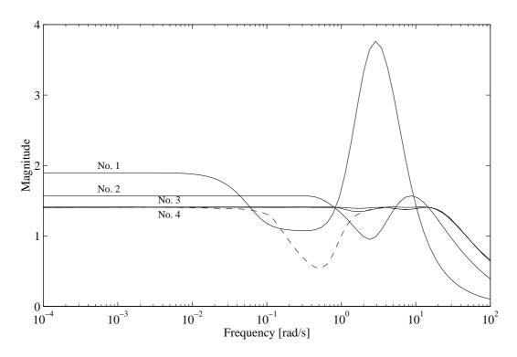
Figure 4.2: Results from D-K iteration on the C.D. player servo. Shown are  $\mu_{\tilde{\Delta}_{\mathbf{c}}}\left(F_l(N(j\omega),K(j\omega))\right)$  for each iteration and also  $\mu_{\tilde{\Delta}}(F_l(N(j\omega),K(j\omega)))$  for the final complex  $\mu$  controller  $K_{\mu_c}(s)$ .
