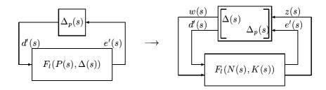
Figure 2.7: Block diagram structure for robust performance check. The perturbation structure is augmented with a full complex performance block  $\Delta_p(s)$ .
