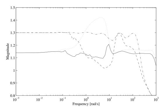
Figure 4.8: Results from  $\mu$ -K iteration on the water tank system. Shown are  $\mu_{\tilde{\Delta}}\left(F_l(N(j\omega),K(j\omega))\right)$ (dashed and solid) and  $\mu_{\tilde{\Delta}_c}\left(F_l(N(j\omega),K(j\omega))\right)$  (dash-dotted and dotted) for the initial (complex  $\mu$  optimal) and final mixed  $\mu$  optimal controller respectively.
