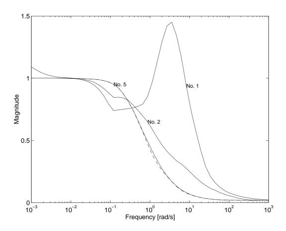
Figure 4.7: Results from D-K iteration on the water tank system. Shown are  $\mu_{\tilde{\Delta}_c}(F_l(N(j\omega),K(j\omega)))$  for iteration 1, 2 and 5 and also  $\mu_{\tilde{\Delta}}(F_l(N(j\omega),K(j\omega)))$  for the final complex  $\mu$  controller  $K_{\mu_c}(s)$ .
