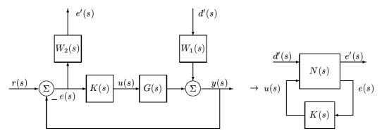
Figure 2.3: Nominal performance problem. Augmented closed loop system and corresponding  $2 \times 2$  block problem.
