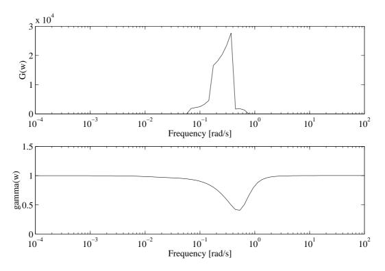
Figure 4.4: G scalings to be fitted in G,D-K iteration (top) and  $\gamma$  scalings to be fitted in  $\mu$ -K iteration (bottom).
