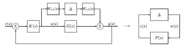
Figure 2.4: Closed loop system with additive perturbation.  $P(s) = W_{u1}(s)K(s)(I + G(s)K(s))^{-1}W_{u2}(s)$ denotes the transfer function "seen" by the perturbation  $\Delta$ .
