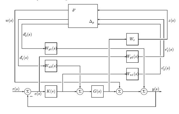
Figure 4.1: Control problem set-up for the C.D. servo drive.
