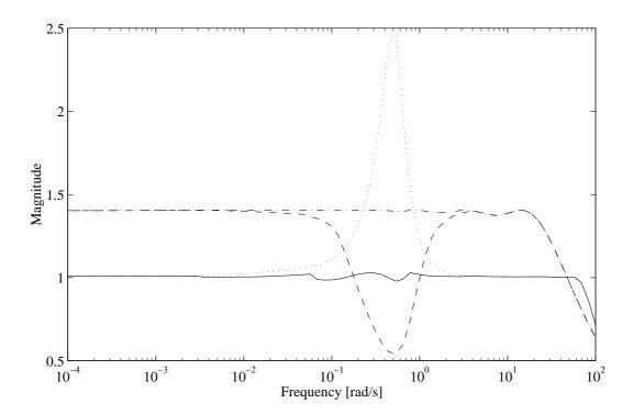
Figure 4.3: Results from  $\mu$ -K iteration on the C.D. player servo. Shown are  $\mu_{\tilde{\Delta}}\left(F_l(N(j\omega),K(j\omega))\right)$  (dashed and solid) and  $\mu_{\tilde{\Delta}_c}\left(F_l(N(j\omega),K(j\omega))\right)$  (dash-dotted and dotted) for the intial (complex  $\mu$  optimal) and final mixed  $\mu$  optimal controller respectively.
