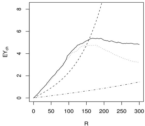
**Fig. 5** Expected connectivity hops versus radio range for different processes: ON/OFF process with high traffic (solid), Poisson process with high traffic (dashed), ON/OFF process with low traffic (dotted), and Poisson process with low traffic (dashed/dotted).
