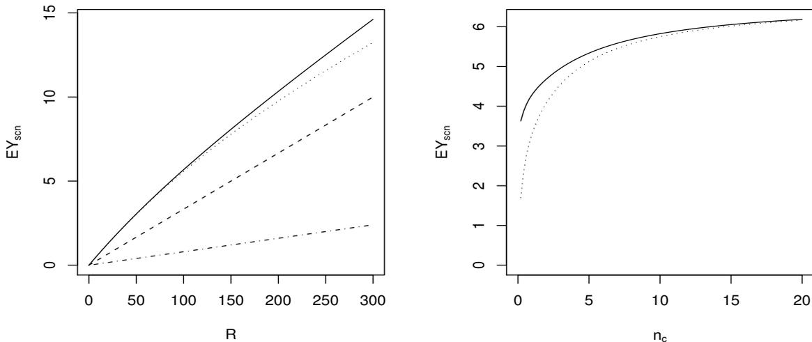
**Fig. 2** Left: Expected single-hop connectivity number versus radio range for different processes: ON/OFF process with high traffic (solid), Poisson process with high traffic (dashed), ON/OFF process with low traffic (dotted), and Poisson process with low traffic (dashed/dotted). Right: Expected single-hop connectivity number versus  $n_c$  for ON/OFF process with high traffic (solid) and low traffic (dotted) for a radio range  $R = 100m$ .
