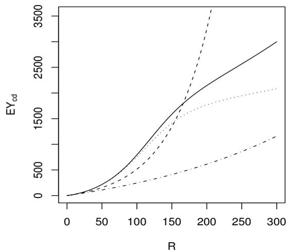
**Fig. 4** Expected connectivity distance versus radio range for different processes: ON/OFF process with high traffic (solid), Poisson process with high traffic (dashed), ON/OFF process with low traffic (dotted), and Poisson process with low traffic (dashed/dotted).
