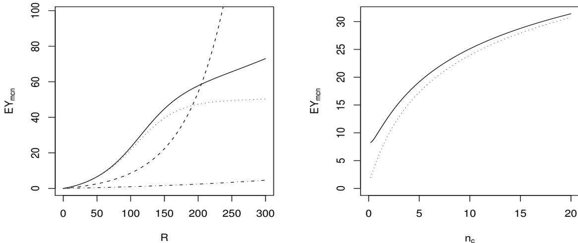
**Fig. 3** Left: Expected multi-hop connectivity number versus radio range for different processes: ON/OFF process with high traffic (solid), Poisson process with high traffic (dashed), ON/OFF process with low traffic (dotted), and Poisson process with low traffic (dashed/dotted). Right: Expected multi-hop connectivity number versus  $n_c$  for ON/OFF process with high traffic (solid) and low traffic (dotted).
