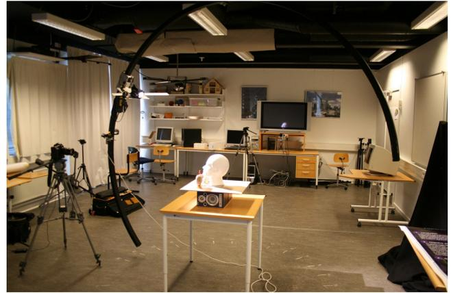
**Figure 2: The actual sphere gantry on the lab. Unfortunately the rig is not motorized so it is manually moved during acquisition.**
