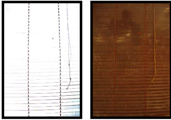
Figure 9. Retroreflective microprisms window blind
