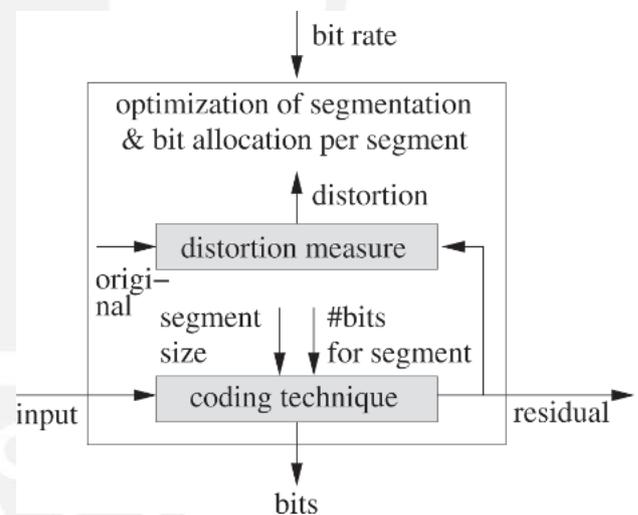
Fig. 2. Segmentation and bit allocation over segments.
