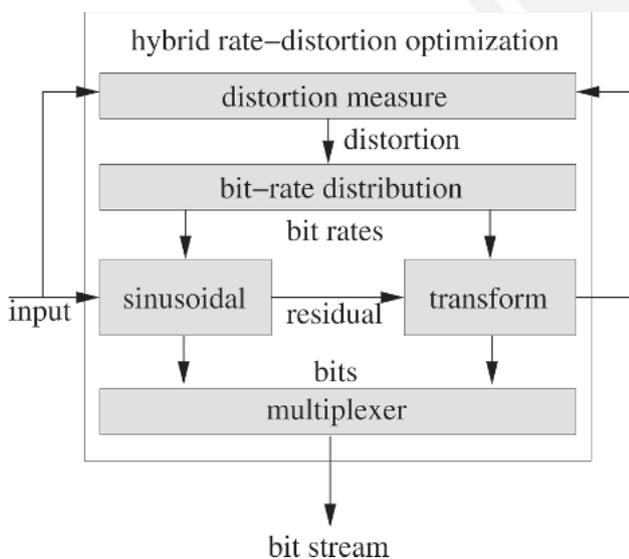
Fig. 1. Operational RD optimized hybrid coding framework.
