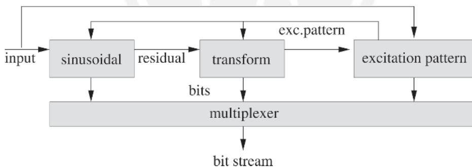
Fig. 4. Illustration showing position of excitation pattern coding.
