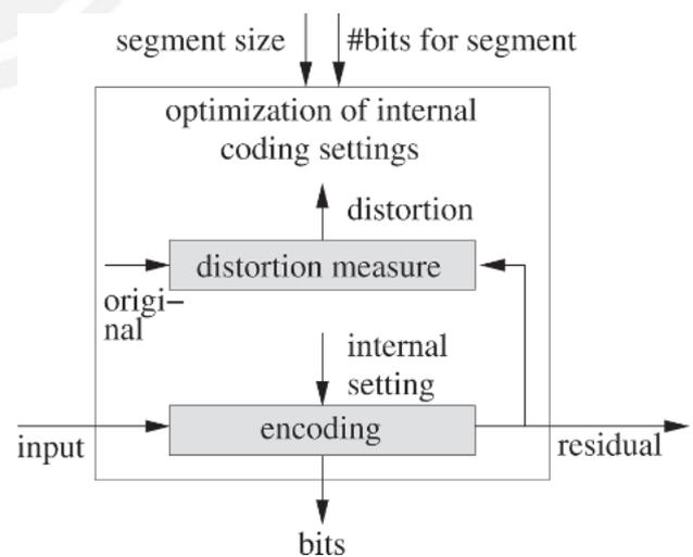
Fig. 3. Internal RD optimization of coding techniques.
