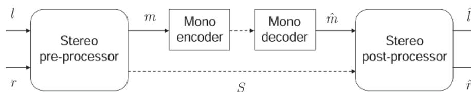
Fig. 7. Stereo coding using pre- and postprocessing techniques. — signals; --- parameter bit streams.  $l$ : left channel;  $r$ : right channel;  $m$ : time- and gain-matched sum of  $l$  and  $r$ ;  $\hat{m}$ : decoded sum of  $l$  and  $r$ ;  $\hat{l}$ : decoded left channel;  $\hat{r}$ : decoded right channel;  $S$ : stereo extension bit stream.
