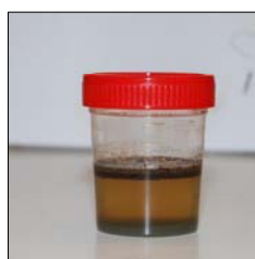
Figure 5. Oil, water and salts after the reactor loop
