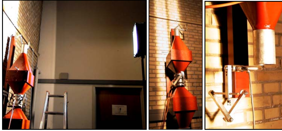
Figure 19. Hot-sphere anemometer in the jet-wind tunnel lit with the lamp imitating solar radiation.
