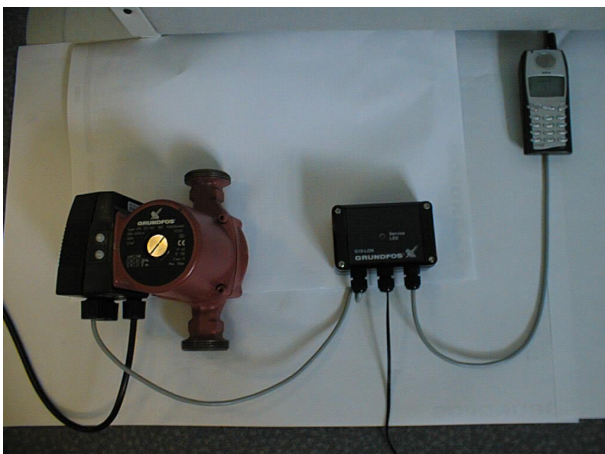
Fig. 6. Pump system, client and phone
