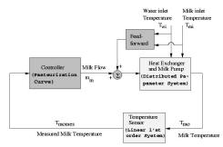
Figure 5: The control structure for the pasteurization system.
