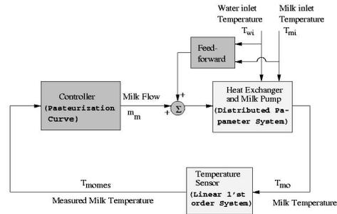
Figure 5: The control structure for the pasteurization system.
