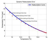
Figure 4: Pasteurization error caused by milk flow variations.
