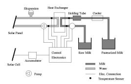
Figure 1: The pasteurization process
