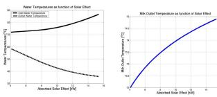
Figure 3: In- and outlet water temperatures versus absorbed effect (left) and milk outlet temperature versus absorbed effect (right).
