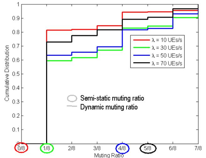
Fig. 6. CDF of the muting ratio for semi-static muting ratio and dynamic muting ratio solutions.
