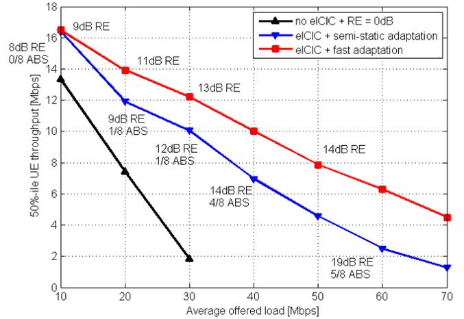
Fig. 4. 50%-ile user throughput as a function of the average offered load with no eICIC, eICIC and eICIC with fast muting adaptation.
