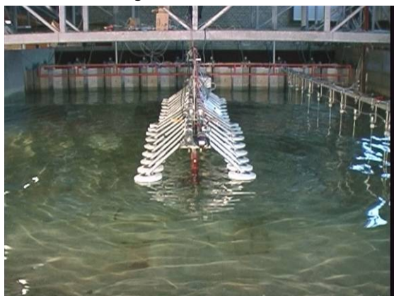
Figure 2. Scale 1:40 converter at Aalborg University (left), and scale 1:10 converter at Nissum Bredning (right).
