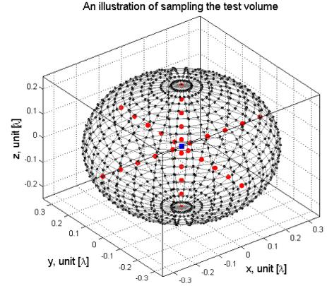
Figure 1. An illustration of different ways to sample the test volume. Blue mark denotes the test volume center. One way is to select locations  $u$  and  $v$  from three orthogonal axes (red marks), as shown in [10], [11]. Another way is to select locations  $u$  and  $v$  on the surface of test volume which are directly opposite each other (black marks).
