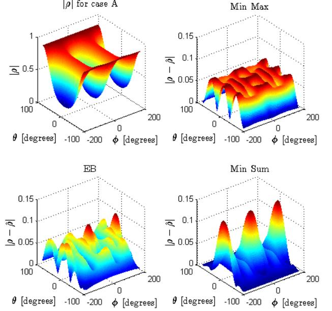
Figure 3. Target spatial correlation  $|\rho|$  between antenna  $u$  and  $v$  on the surface of the test volume for case A and associated reconstruction results  $|\rho - \hat{\rho}|$  with different algorithms.
