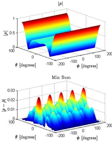
Figure 5. Target spatial correlation  $|\rho|$  between antenna  $u$  and  $v$  on the surface of the test volume for case D and associated reconstruction results  $|\rho - \hat{\rho}|$  with Min-Sum algorithm.
