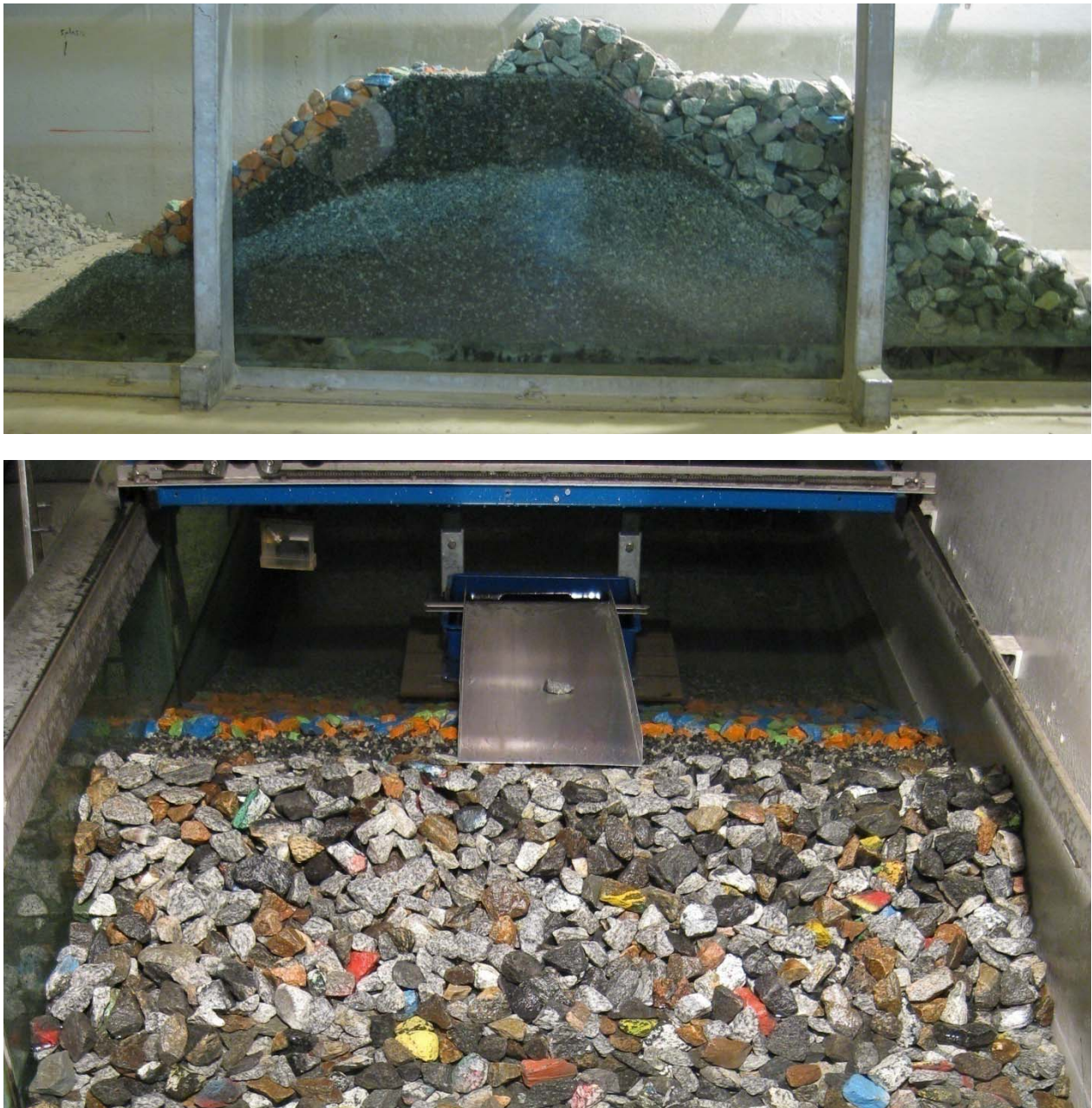
Figure 2: Pictures of the cross section and the overtopping ramp and tank.
