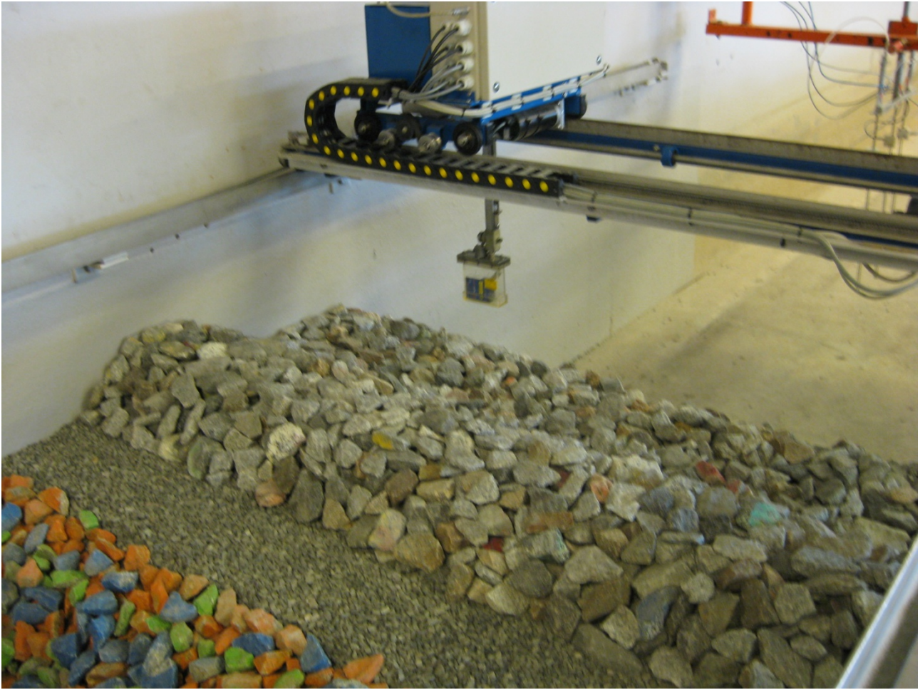
Figure 3: Pictures of laser profiler and the initial cross section viewed from the harbour side.
