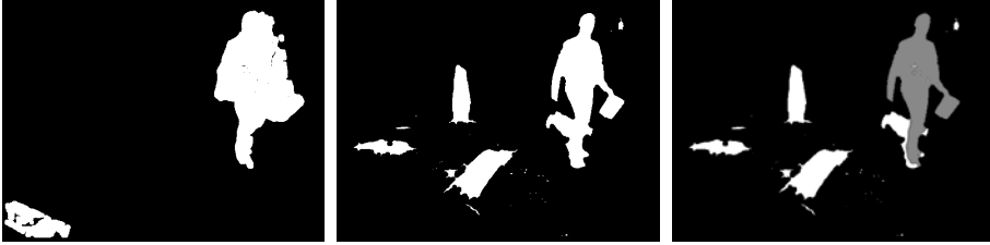
Fig. 5. Left: thresholded disparity difference (change in depth). Center: thresholded color difference (change in color). Right: changes classified into moving object (grey) and shadow candidates.
