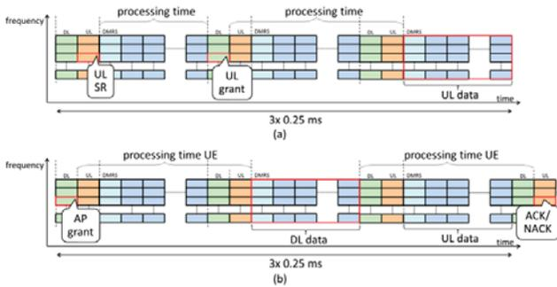
Figure 2. RTT for scheduling (a) and HARQ (b).
