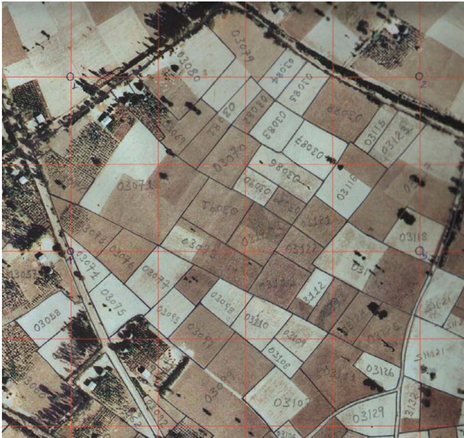
Figure 2: Orthophoto used as a field work map sheet with a georeferenced grid. The map shows the delineated parcel boundaries and parcel identification numbers. (Ethiopia).
