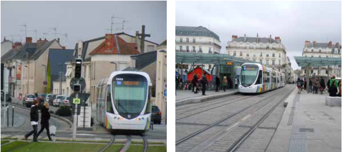
Figure 6: The two parts of the light railscape where the light rail operates on the APS ground power supply system (see third line placed in-between tracks): the light rail in the small village of Avrillé (right) and the central city shopping square in Angers “Place du Ralliement” (left) – making two diverse districts equal (Photos by author).
