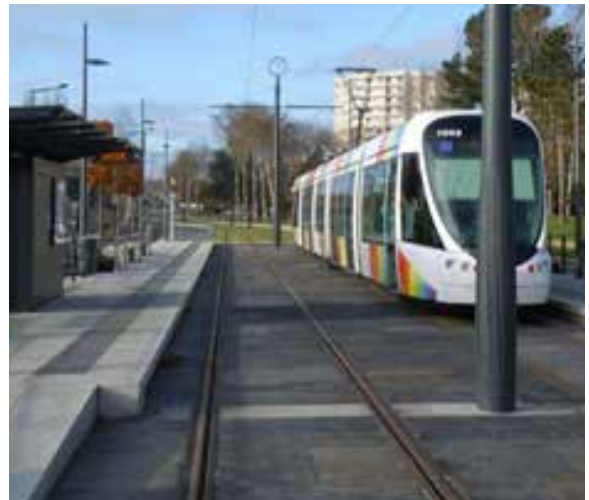
FIGURE 14: The local gained material slate is used at the stations, also to symbolize the local identity in the project. The colours of the station are in the same as the pavement, and the paper bins and the lamp post have same finesse. Notice the mast in the background with the circle and a T for 'Tram' in the middle - a landmark to indicate the prescense of a stop. (Photo by author).
