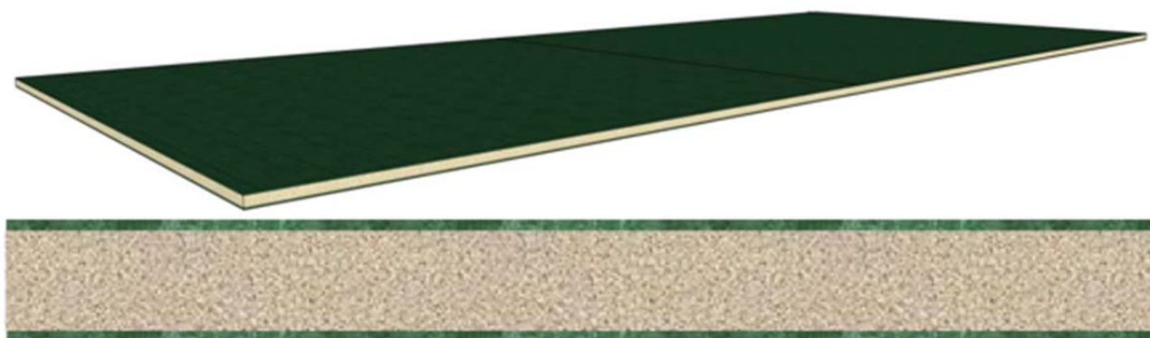
Figure 2.4: Illustration of a carbon FRP composite panel (top) and a close-up on the core and the fibre reinforced laminates (bottom). (Evegren and Rahm 2012, p 11)
