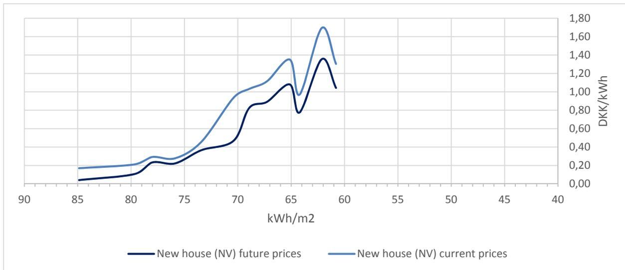
Figure 2.4. Costs for heat savings in new buildings with natural ventilation
