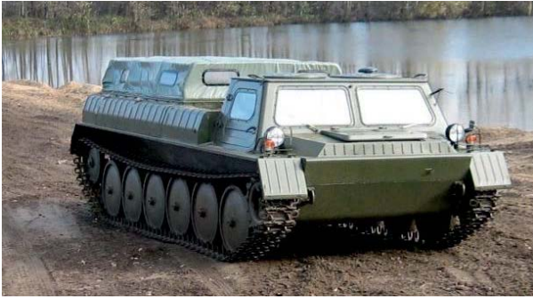
Figure 2. GAZ-71, the all-terrain vehicle on tracks, 1968 (image source: http://www.vsevezdehody.ru )
