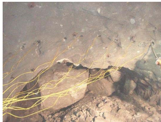
Figure 6: Eyebrow break from AL992 by using double-primer placement with electronic detonators.
