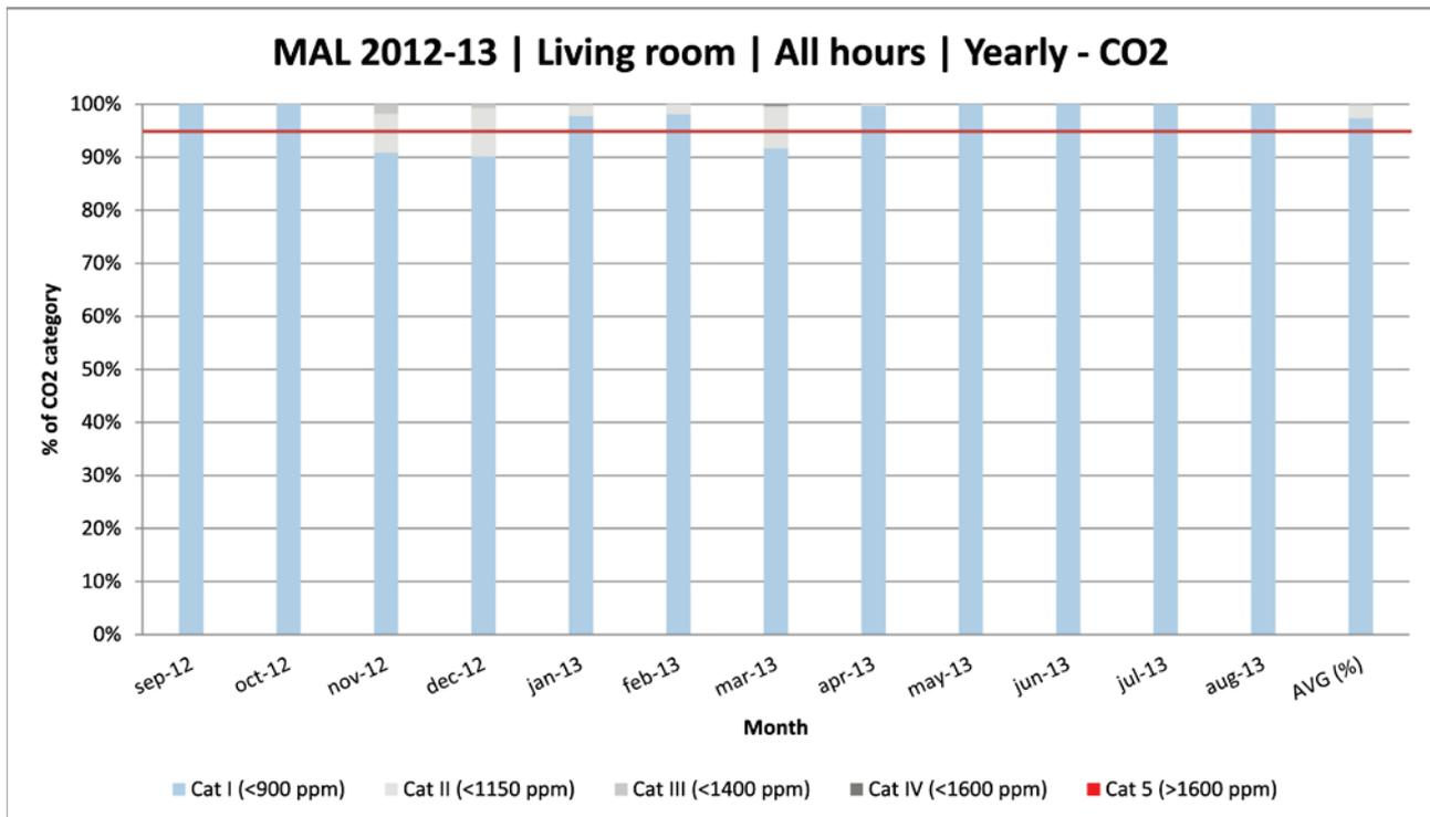
**Figure 4.** CO<sub>2</sub> levels in living room divided into categories as defined in Active House Specification. Values are the absolute, measured values.
