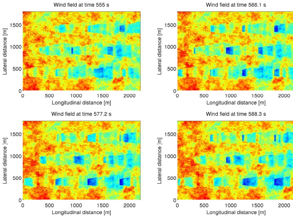
Figure 10: Evolution of the wind field including wakes.
