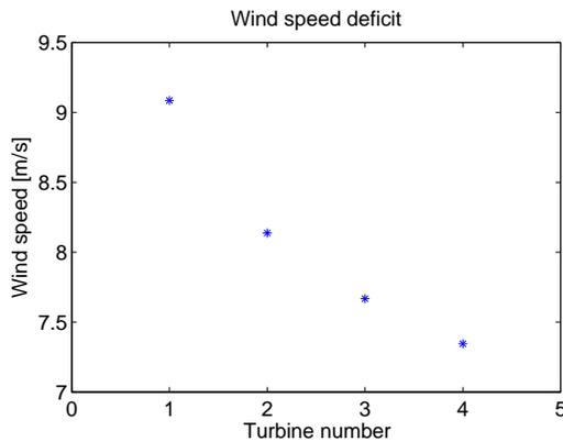
Figure 11: Average wind speed at turbines 1 to 4.
