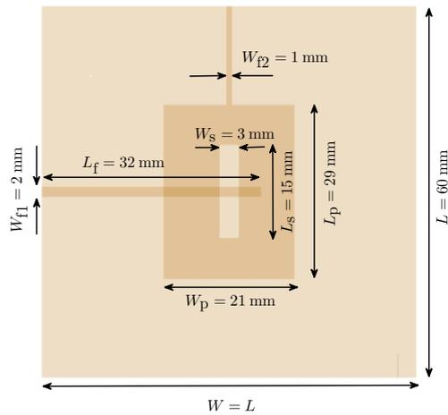
Fig. 3. Dimensions (in mm) of one of the 3 patches (bottom view) comprising the proposed full-duplex MIMO antenna system.
