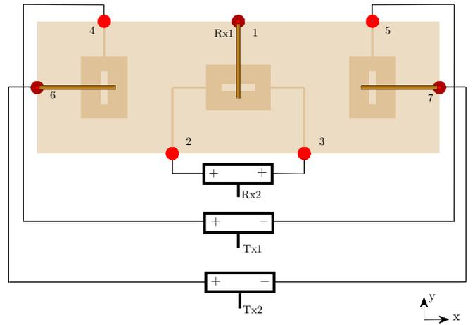
Fig. 2. Symmetric topology of three side-by-side patch antennas (bottom view) showing the out-phasing and the in-phasing of the Tx and the Rx signals for Tx signal cancellation at the Rx.
