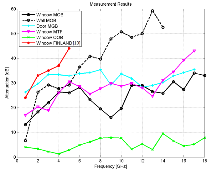
Fig. 6. Measured attenuation for the different scenarios in the range from 800 MHz to 18 GHz.
